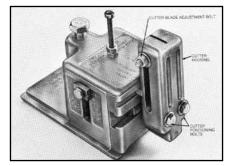
**5.** Set belt cutter (cut off) blade by loosening the two bolts on the belt cutter housing. Starting from the centermost position, move the housing toward the belt end until top alignment mark lines up with fastener number to be installed. Retighten bolts.
