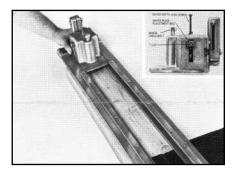
3. Warning: Skiver and cutter blades are unguarded and extremely sharp. On a woven belt, calculations for belt thickness should be made in center of belt. Set skiver blade by loosening bolts on either side of skiver head and aligning T-lug on 1/16" marks (these marks are approximate and may vary slightly due to belt cover hardness) for depth of cut. Retighten bolts and put skiving head on opening in track with skiver blade toward belt edge.
