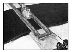
6. Loosen blade-depth and lower blade until it contacts wood base. Connect winch cable to skiver head and crank it across. Silicone spray on belt will help. Retract blade and remove skiver head and track from belt. Repeat operation on opposite end of belt.
