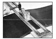
4. Hook winch cable on ½" bolt on top of skiver and crank winch to draw skiver across the belt. Spray Flexco® silicone lubricant on track and belt. After skiver cuts about six inches, stop and nail the skived flap back in place to keep flap from jamming in skiver. Complete the skive. Adjust skiver blade back up into skiver head and return skiver head to start position.
