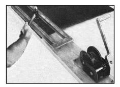
2. Lay a clear, (free of knots or nails) straight wooden plank, minimum 2" x 8", on a firm surface crosswise under the belt and under squared line. Nail winch on one end. Be sure winch handle operates freely. Nail track along squared line or square edge of belt (use every hole on both sides of track over belt) with opening for skiver head at opposite end from winch. Use No. 16D coated nails provided. Reset all nails.
