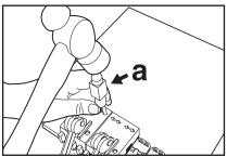
**9.** Starting with the center fastener plates, strike (a) staple driver with a 0.5 kg (1 lb.) hammer. Do not overdrive staples. Raise cam lever(s) to remove tool.
