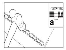
**12.** Set fastener strip flat on ST-28 setting plate. Strike top-side of fasteners and staples with firm hammer blows. Move back and forth across fastener strip until (a) staples clinch. Avoid hitting fastener loops. Repeat steps 1-12 on other belt end.
