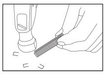
**6.** To insert staples without the dispenser, separate staples by tapping lightly with hammer or "crumble" the sticks by hand.
