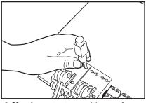
8. Very important — position staple driver in applicator and push staples down by hand until staples contact belt. Otherwise staples can wander when driven by hammer.
