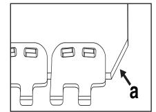
**13.** Using (BN-1) Belt Nippers, (a) notch trailing edge of belt only. Notch at an angle.
