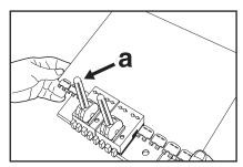
**3.** Place the installation tool on the center of the fastener strip. (a) Cam lever(s) should be up.
