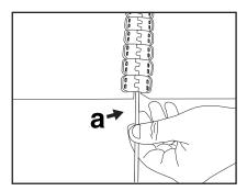
**14.** Bring belt ends together and (a) insert hinge pin. If retaining washer is used, crimp with pliers. Splice is complete.
