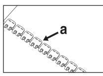
**2.** Place belt on solid surface for support. Center fastener strip, equal distance from the belt ends. (a) The word "Alligator" should be facing up.
