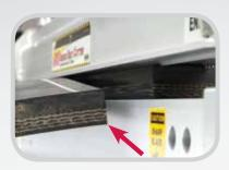
The single-sided clamp feature allows the cut belt to fall free on one side, eliminating the need for the blade to cut through two clamped surfaces, reducing operator effort.
