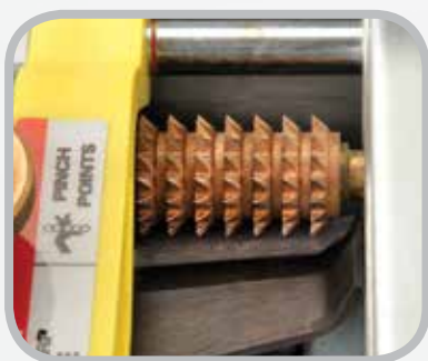
Front drive rollers aggressively grip belt at the start of the skive to prevent slippage.
