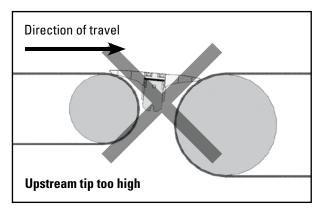
**WARNING:** This is an example of an incorrect installation. The transfer plate is installed above the head pulley and tilted downstream, this will create interference with the flow of material between the conveyors.
