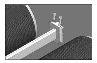
7. After verification that the tack weld has occurred, remove the socket head screws from the mounting brackets and lift the assembly with the front plates out of the transfer leaving only the back plates in place and finish welding the back plates with a 25 mm (1") bead on two sides of the plate.
