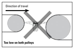
**WARNING:** This is an example of an incorrect installation. The transfer plate is installed below the correct placement position, it will cause the flow of material to choke between the conveyors.
