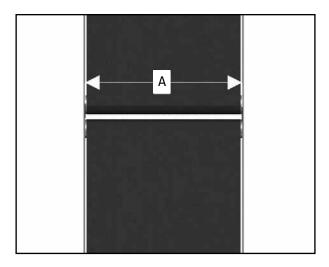
Once you have determined dimension "A" (overall width of the conveyor), select the STP gauge key that properly fits in between the pulley where the transfer plate will be installed.
