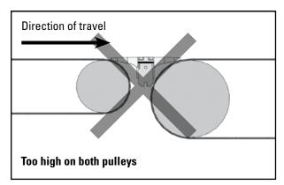
**WARNING:** This is an example of an incorrect installation. The transfer plate is installed above the correct placement, it will interfere with the flow of material.
