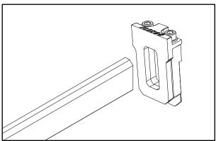
**4.** Slide one mounting bracket assembly onto each end of the bar. Ensure that the front plate is located in the center of the back plate slot to allow for maximum STP adjustment.
