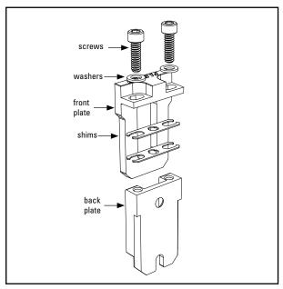
3. Stack two shims on top of back plate of each mounting bracket. Using socket head screws and washers, attach front plate to the back plate, ensuring that the shims are in place. Align the edges of the front and back plates so that the vertical edges are parallel. Tighten screws to compress shims, ensuring no interference with the pole end.
