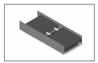
5. Position the support bar with segments and mounting brackets into the transfer gap. The resting position of the bar and the brackets should be similar to the one identified by the STP KEY location in SECTION 3. Ensure segments are not resting on top of the pulley crown or in the tapered section.
