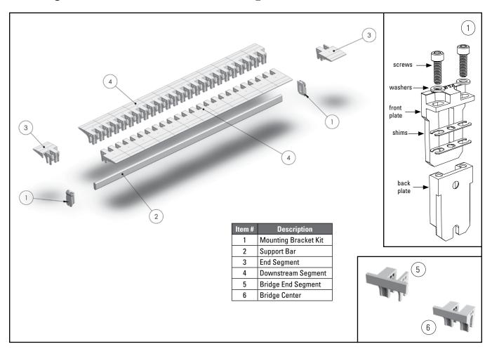
Flexco Segmented Transfer Plates are designed to absorb the damage of a foreign object and protect the belt from any injury while maintaining product flow. The transfer plate was designed to be compatible with polybags, nylon bags, small packages, and general parcel and material.
