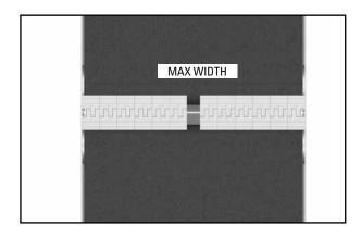
11. From the center of the bar, push the segment pairs toward the ends of the bar, ensuring that they are tightly butted against each other. Measure the gap that remains between the center-most segments to determine the size of the final segment set.
