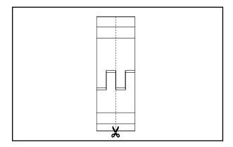
**CAUTION:** Do not trim more than half off a segment pair or 38 mm (1.5"). It is recommended to trim both segments of a segment pair while they are nested to ensure consistent segment.
