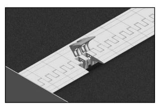
12. Install the last (trimmed) segments into the remaining gap. If the support bar does not appear centered in the gap between pulleys, loosen the socket head screws and adjust the transfer. 3 mm (1/8th inch) total adjustment is available.
