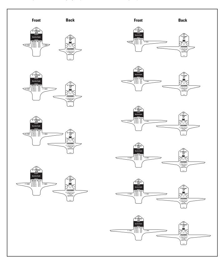
Determining the correct transfer plate item number and its location is a process of trial and error. We recommend that you prepare for the measurement process with an STP gauge key and measure the gap between the pulley until you achieve the correct fit between the STP gauge key and the pulleys. The following example will explain you the proper way to use the STP gauge key and how to select the correct Segmented Transfer Plate item code for ordering.
