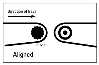
**1. Horizontal to Horizontal Conveyors** Both conveyors are aligned and the belts have the same direction of travel. This arrangement is usually level.
