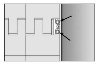
**14.** Once all adjustments are made, secure the screws on both sides of Segmented Transfer Plate assembly with a thread locking agent.
