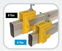
6 ton clamps are available for belts up to 1800 mm (72") wide and up to 50 mm (2") thick, while the 8 ton clamps are available for belts up to 2400 mm (96") wide and up to 55 mm (2 1/4") thick.
