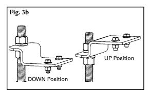
4. **Check performance.** Run the belt and check that the plow runs smoothly and has an effective cleaning action. A final adjustment may be required. To raise or lower the unit, adjust the nuts against the mounting bracket up or down.
