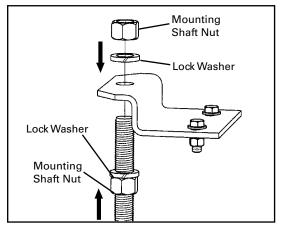
3. **Install the mounting brackets on the mounting shafts.** Put a lock washer onto each mounting shaft and slide the mounting brackets on (Fig. 3a).
