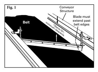
1. Position the plow frame on the conveyor. Slide the plow onto the belt in the selected location. Check for structure interference at both ends where the mounting brackets will be attached to the structure (Fig. 1).
