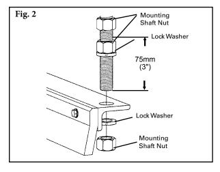
2. Attach the mounting shaft to the plow frame. Thread two mounting shaft nuts up the mounting shaft to expose 75mm (3") of thread past the nut. Next place a lock washer against the lower nut and slide the mounting shaft down through the hole in the plow frame (Fig. 2). From the bottom side of the plow frame place a lock washer and mounting shaft nut on the mounting shaft and tighten. Repeat on opposite side.
