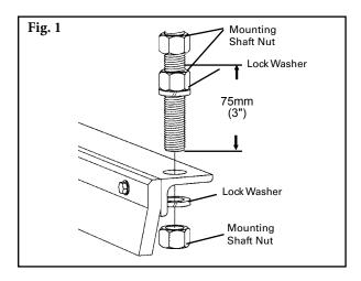
1. **Loosen mounting shaft nuts.** The bottom two mounting shafts nuts on both sides of the plow should be loosened so that the worn blade will have no tension to the belt (Fig 1.)
