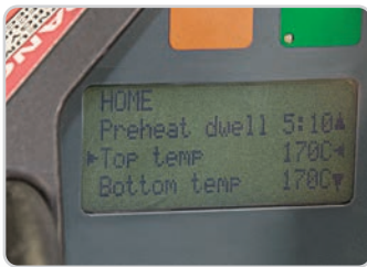
Ability to set independent temperatures of top and bottom heating elements to ensure optimal splice.
