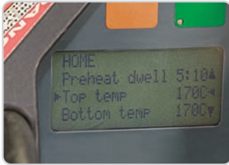
Ability to set independent temperatures of top and bottom heating elements to ensure optimal splice.
