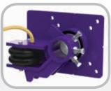
**Compression Spring:** Maintaining proper tension is key to maximizing blade life and cleaning performance. The simple but effective compression spring design from Flexco allows anytime tension verification and can be adjusted without waiting for a shutdown. Flexco also offers other tensioners such as air and nitrogen that can offer premium performance options.
