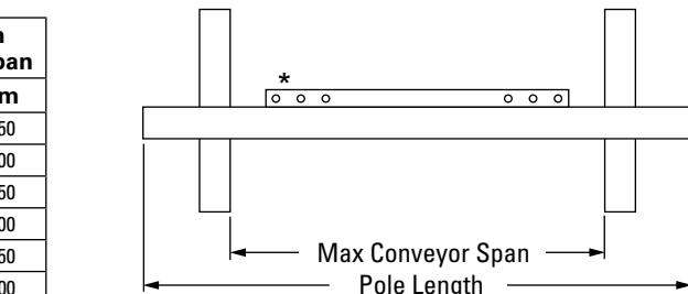
\*Each pole size can be used with a blade size either belt width minus 150mm (6"), belt width minus 300mm (12"), or belt width minus 450mm (18").
