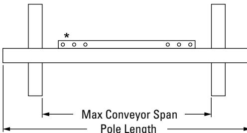
\*Each pole size can be used with a blade size either belt width - 6", BW -12", BW -18", BW -24", BW -30", BW -36"
