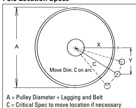
A = Pulley Diameter + Lagging and Belt
