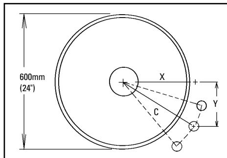
1. **Determine the given location dimensions and define the change needed.** After laying out the given X & Y dimensions, determine the distance of the modification required for adequate clearance of the pole and tensioning system. (In the example we decide to lower the pole 50mm (2") to clear the support structure).
