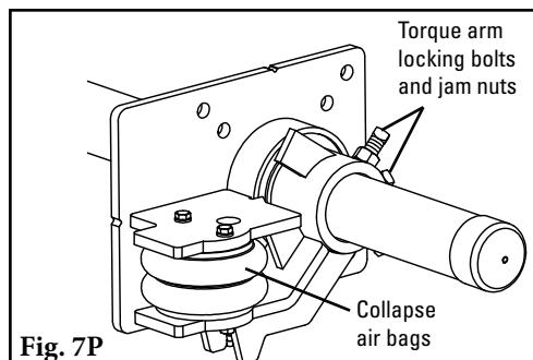
**NOTE:** PAT Tensioners are shipped with the air bags and torque arms attached to the mounting bases.
