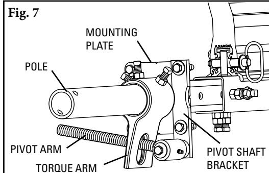
**8S. Reassemble the spring assembly.** Slide the spring, washer and bushings onto the pivot arm and turn the two adjusting nuts so about 6mm (1/4") of the pivot arm is exposed above the nuts (Fig. 8).
