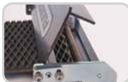
Closed cover clamps belt tightly in place to allow for uniform skive
