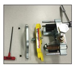
Step 2. Remove handle and plastic fence assembly.
