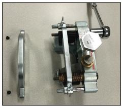
Step 3. Attach metal fence, handle and securely hand tighten remaining screws.
