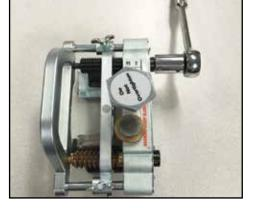
Step 3. Attach metal fence, handle and securely hand tighten remaining screws.
