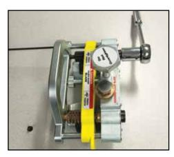
**Step 1.** Loosen existing handle screws with a 5/32" hex wrench and set aside.
