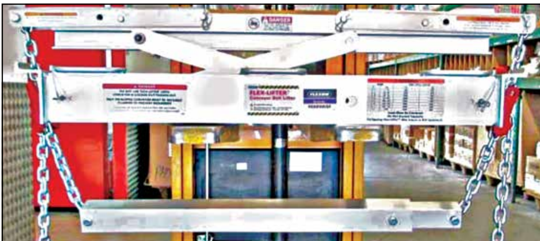
Fig. 35 Lifting rod hanging from the chain
