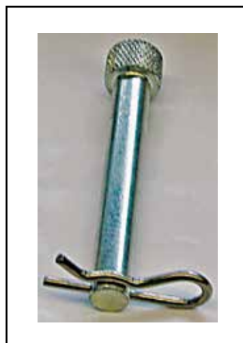
Fig. 12 Blade pin with cotter pin on the troughing belt
