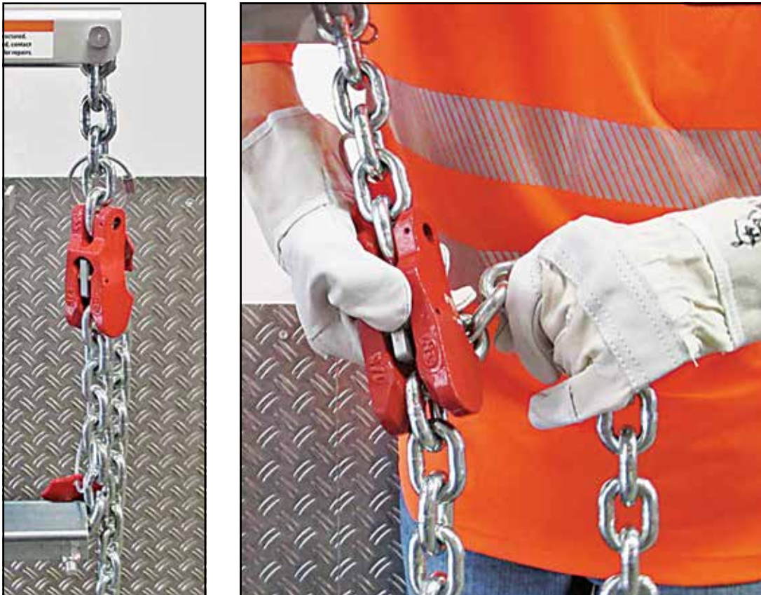
Fig. 34 Unhooking the chain from the lifting rod
