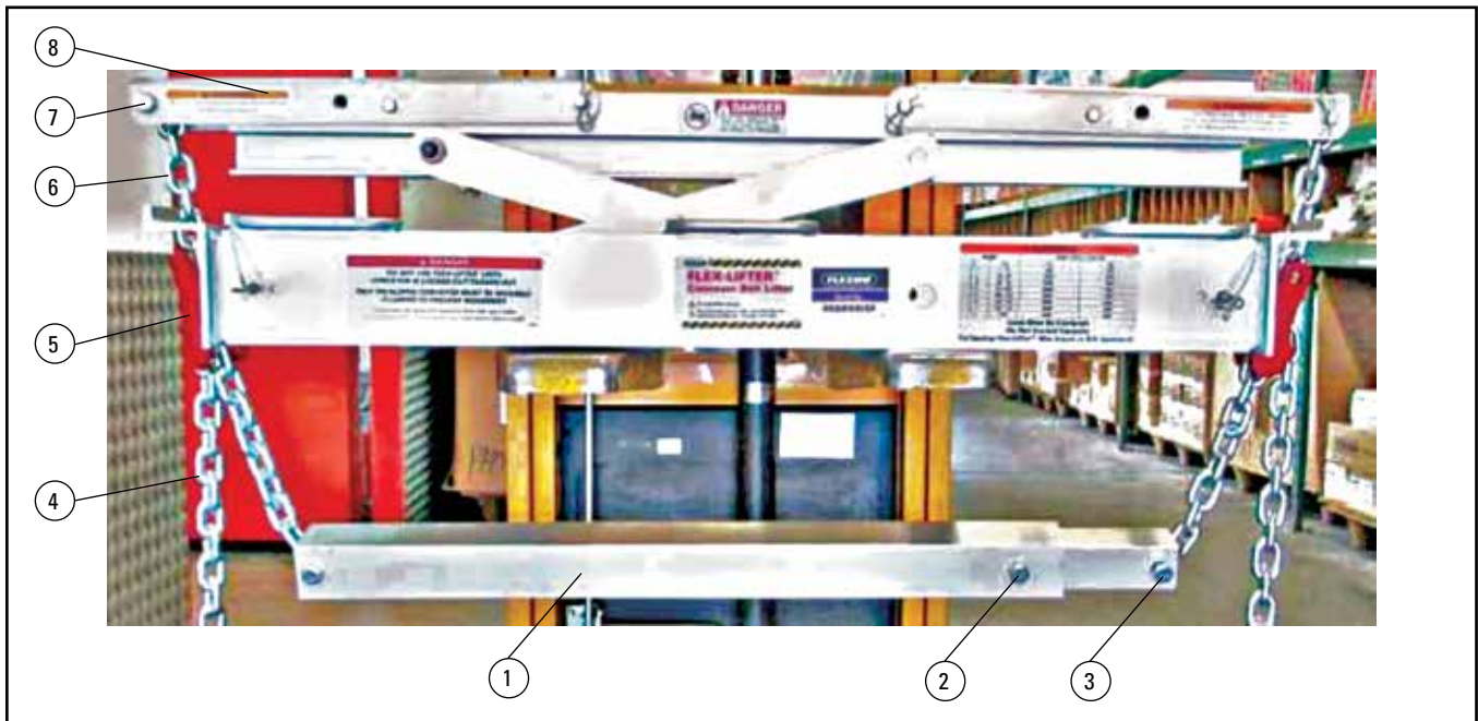
Fig. 6 Flex-Lifter with lifting rods for return belts
