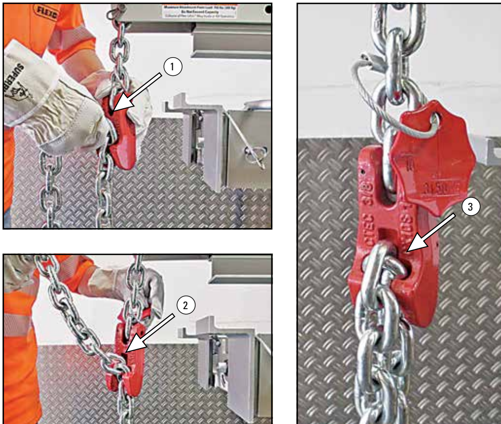
Fig. 33 Attaching the chain to the lifting rod
