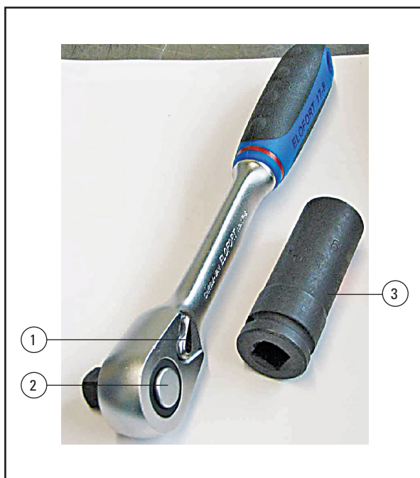
Fig. 13 Nut driver with ratchet example
