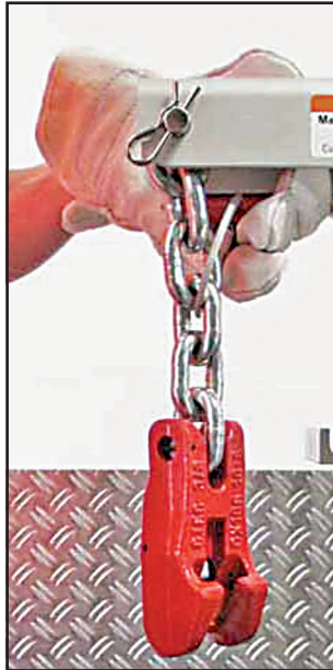
Fig. 31 Attaching short chains
