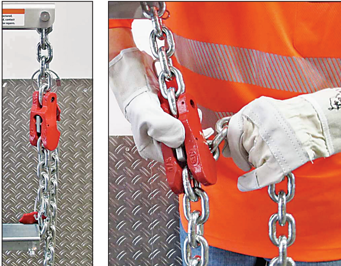
Fig. 34 Unhinging the chain from the lifting rod
