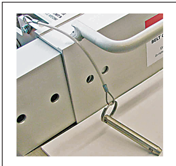
Fig. 11 Blade pins on the extendable foot sections
