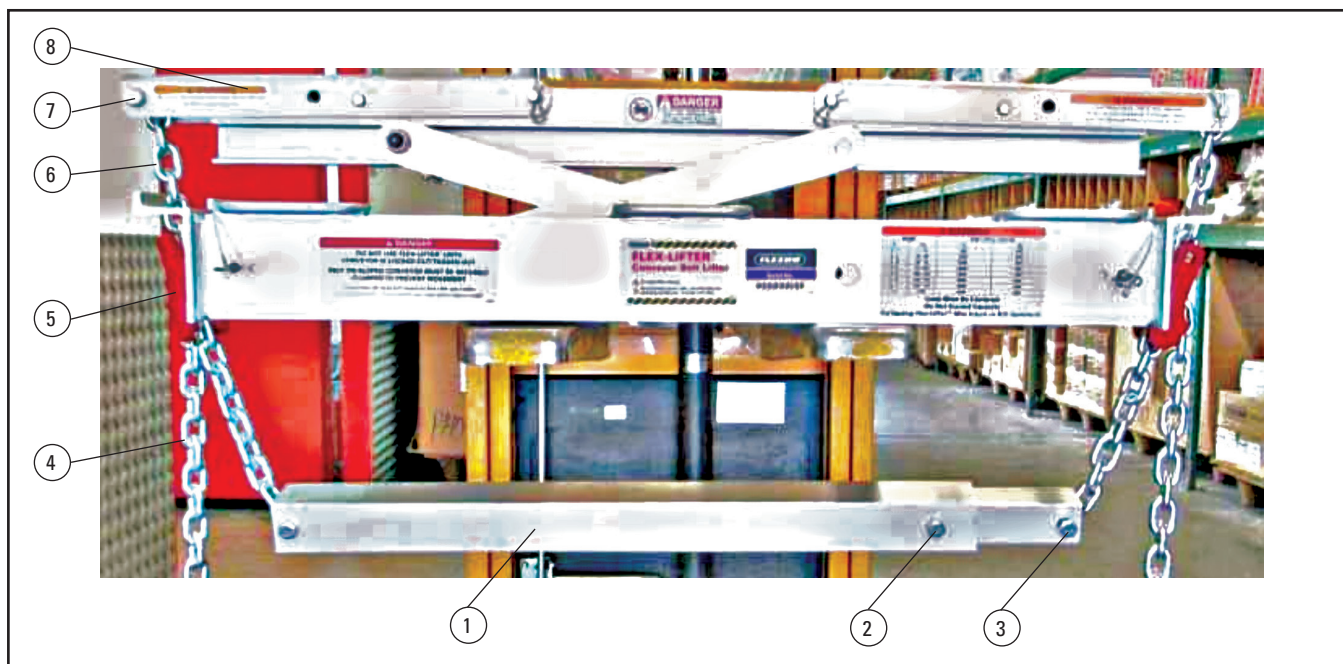
Fig. 6 Flex-Lifter™ with lifting rods for return belts
