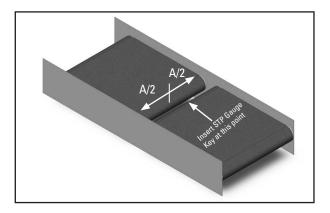
When inserting the STP gauge key, you should have a minimum distance between the top of the STP profile and the tangent point of the belt and the pulley of no less than  $\frac{1}{2}$ " (13 mm) in smaller diameter pulleys. For large diameter pulleys, the distance should not exceed 1.5" (38 mm). The bottom corner of the transfer plate plastic segment should have full contact with the belt and the key should rest level to the imaginary line that joins the crowns of the pulleys.
