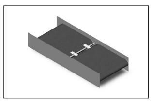
5. Position the support bar with segments and mounting brackets into the transfer gap. The resting position of the bar and the brackets should be similar to the one identified by the STP KEY location in SECTION 3. Ensure segments are not resting on top of the pulley crown or in the tapered section.
