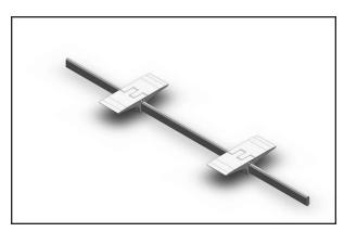
2. Slide one segment pair onto the bar from each end and position each approximately 1/4 of the total bar length from the end so that they do not rest on the top of the pulley crown or on the tapered section.
