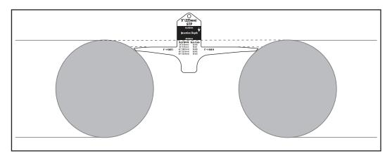
Incorrect placement of the STP Gauge Key, as described in the following examples, could lead to incorrect STP selection. **WARNING:** Incorrect placement of the STP Gauge key will result in erroneous readings and will lead to the selection of the incorrect item code.
