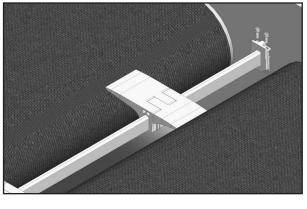
8. Slide the front plates on the mounting bar and replace the shims on top of the back plate. Then set the transfer into position on the back plates. Tighten the two socket head screws at each mounting bracket to secure the system in place.
