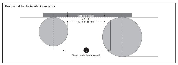
Dimension "B" will be obtained by locating a straight edge between the center lines of the pulleys. The dimension will be obtained by offsetting a parallel line towards the center of the pulley. The total offset should be between 1/2" to 1.5" (13 to 38 mm) below a line between the tangent points on the pulleys for most applications. The "B" dimension should be obtained by measuring the distance between the pulleys where the offset line intersects the outside diameter of the pulleys.
