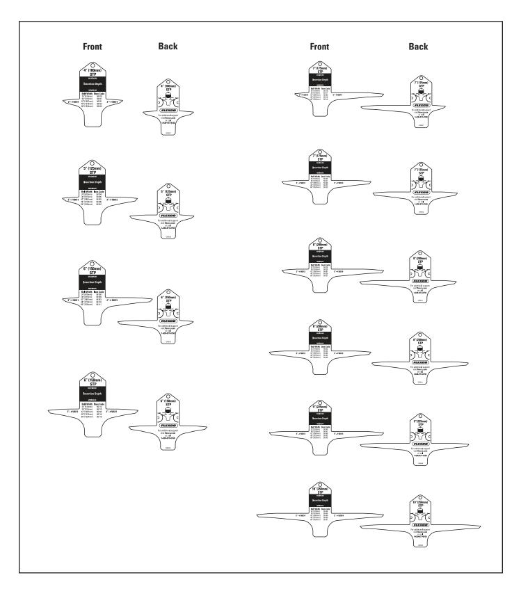
Determining the correct transfer plate item number and its location is a process of trial and error. We recommend that you prepare for the measurement process with an STP gauge key and measure the gap between the pulley until you achieve the correct fit between the STP gauge key and the pulleys. The following example will explain you the proper way to use the STP gauge key and how to select the correct Segmented Transfer Plate item code for ordering.
