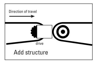
• In the particular case of waterfall conveyor arrangements (incline or decline configurations) there may be gaps where the conveyors meet. Make sure there is adequate structure to mount the transfer plate mounting brackets at the point of installation. If necessary, add a support plate to ensure safe and proper installation of the Segmented Transfer Plate mounting brackets.
