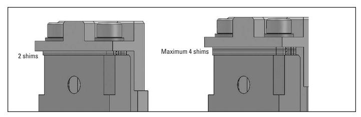
13. By adding or removing shims from the mounting brackets, the transfer can be adjusted up or down a total of 1/8" (3 mm). This should allow adequate adjustment for crowned pulleys or a belt with a profiled top cover.
