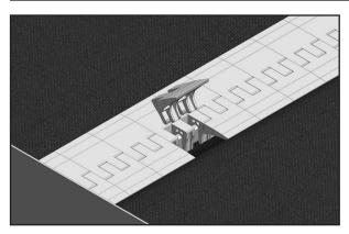
12. Install the last (trimmed) segments into the remaining gap. If the support bar does not appear centered in the gap between pulleys, loosen the socket head screws and adjust the transfer. 1/8" (3 mm) total adjustment is available.
