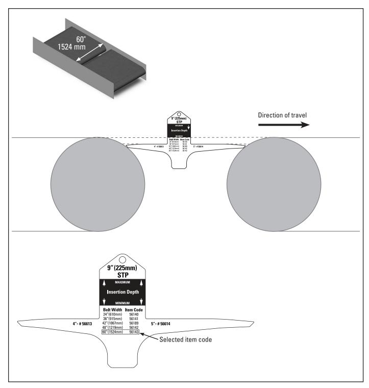
**IMPORTANT NOTE:** In the event that the segment transfer plate requires an offset installation, make sure the short segment is installed upstream (towards the head pulley or against the direction of travel). The downstream plastic segment (long segment) should be installed towards the trailing pulley (direction of travel).
