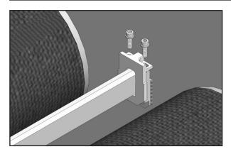
7. After verification that the tack weld has occurred, remove the socket head screws from the mounting brackets and lift the assembly with the front plates out of the transfer leaving only the back plates in place and finish welding the back plates with a 1" (25 m) bead on two sides of the plate.
