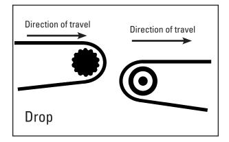
**4. Horizontal to Horizontal Drop Conveyors.** Both conveyors are aligned, but not level and the belts have the same direction of travel. The first belt will feed the second belt. There is a clear drop between the belts.
