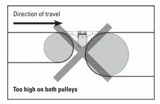
**WARNING:** This is an example of an incorrect installation. The transfer plate is installed above the correct placement, it will interfere with the flow of material.
