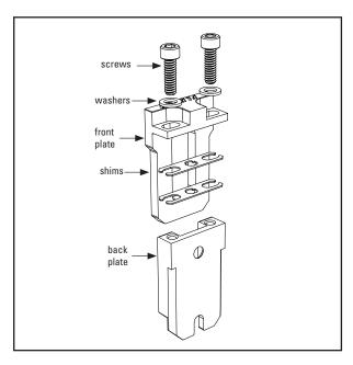
3. Stack two shims on top of back plate of each mounting bracket. Using socket head screws and washers, attach front plate to the back plate, ensuring that the shims are in place. Align the edges of the front and back plates so that the vertical edges are parallel. Tighten screws to compress shims, ensuring no interference with the pole end.
