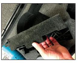
**Step 1.** Remove the cutter. You will see a "raised" foam insert member which the current rail system rests on. Remove that piece. There may be some light adhesive on the bottom of it which secures it in place.
