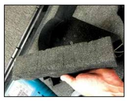
**Step 2.** Take an Exacto knife or extendable razor knife and decrease the thickness of that foam insert by 1/2.
