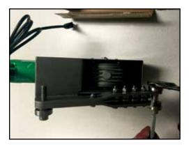
Step 1. Loosen existing rail lock nuts with 8 mm or 5/16" hex and 17 mm box end/crescent wrench. Set aside lock nuts, bearings and washers.
