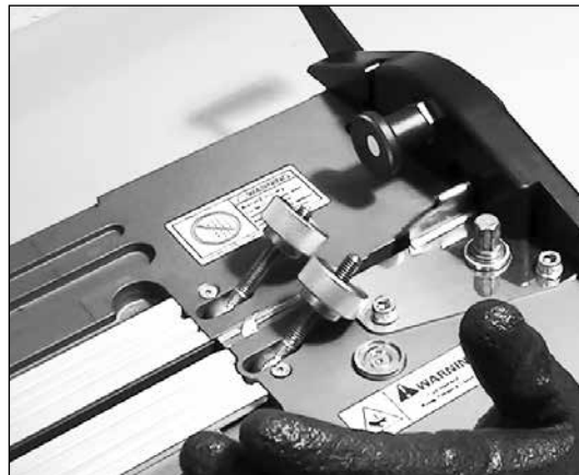
19. Ensure fixed platen is lightly against blade holder.
