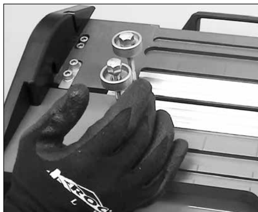
15. Move fixed platen lightly against blade holder.
