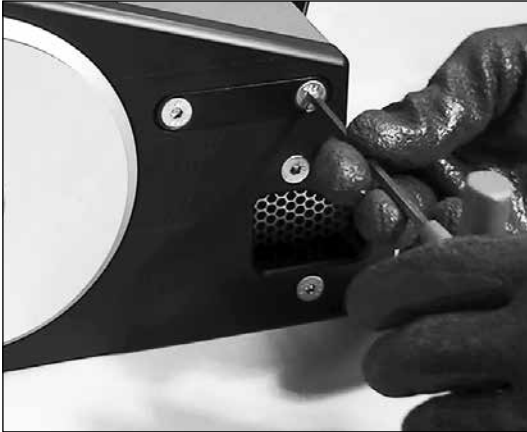
16. Fully tighten two (2) adjacent side platen locking screws.
