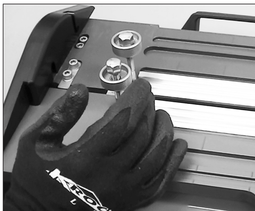
15. Move fixed platen lightly against blade holder.
