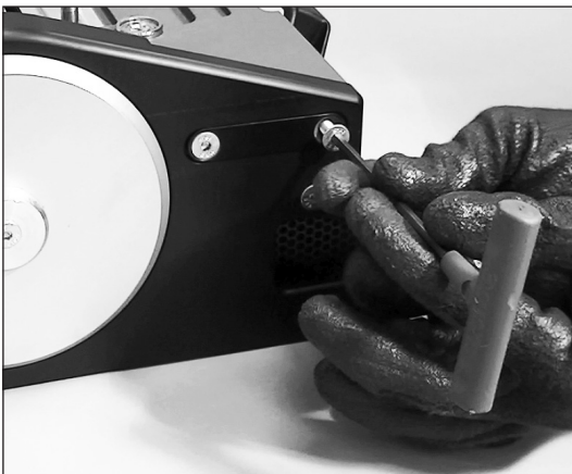
1. Loosen and remove four (4) platen locking screws.
