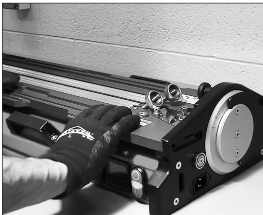
10. Lock actuating disc in cut/load position.
