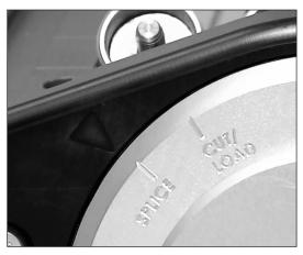
1. Rotate actuator lever to SPLICE position. **Caution!** Emitter is exposed during operation. Use caution to avoid damage.
