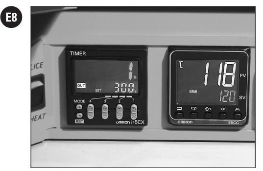
Allow preheat period to expire. A sound tone will be heard at conclusion of preheat cycle. Allow machine and belt to cool to preset "splice start" temperature.
