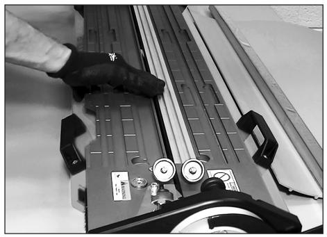
Relocate belt template to opposite platen. Repeat belt end preparation on second belt end (Steps C7 through C16).
