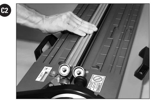
Ensure only one template is installed.
