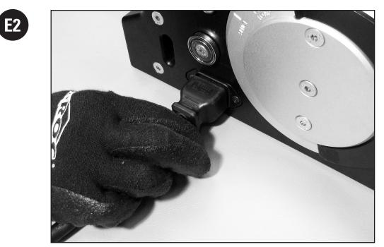
Select proper power cable and plug into machine power inlet.
