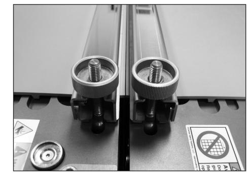
Position actuator lever to permit prepared belt ends to abut. There should be no more than approximately 0.1 mm (.004") gap along entire abutted faces. If gap is greater or uneven, it may be necessary to reprepare belt ends.
