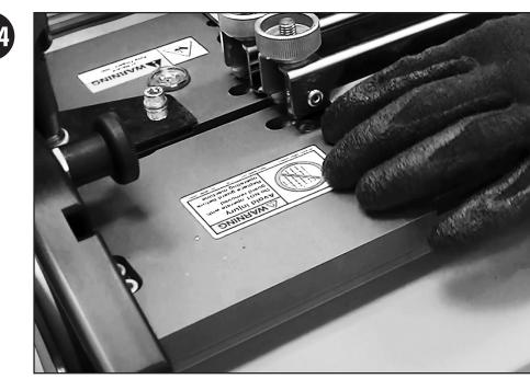
Support belt to prevent belt from "peeling away" during cutting. Failure to comply will result in an uneven cut where blade exits from belt. TIGHTLY CLAMPED side of belt is now prepared for splicing.
