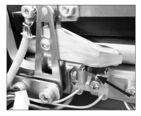
**1.** Using 3 mm allen wrench pull up to reset red button.
