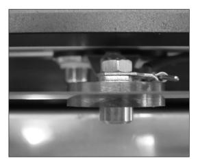
**9.** Ensure emitter is positioned on (or over) emitter support roller. **Note!** Emitter may possess a slight "bow" thus preventing initial contact with support roller. This will relax after several conditioning heat cycles. Ensure emitter is not in contact with thermocouple.
