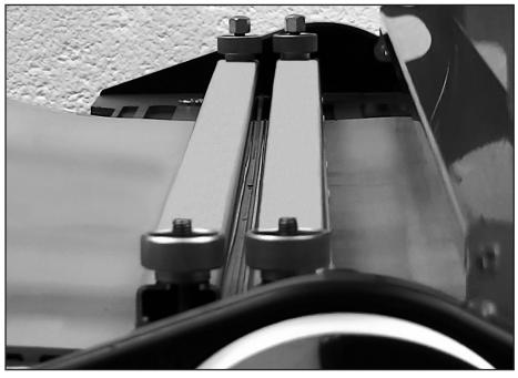
After light signal indicates conclusion of splice process, remove guard. **Caution!** Guard, clamp bars, and clamping thumb nuts remain hot after end of process indication.
