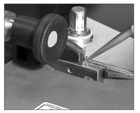
3. Using pliers, remove blade from blade holder.
