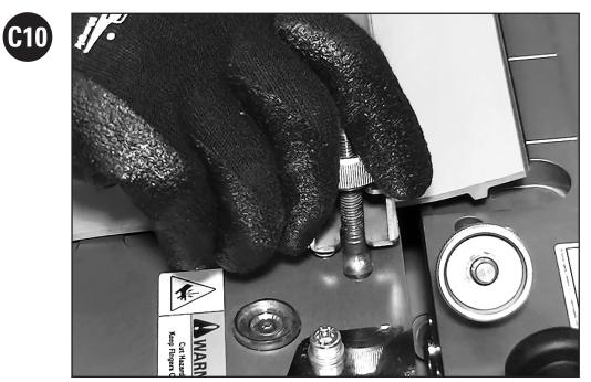
Install one clamp bar tightly over installed belt and template.
