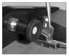
4. Install new blade or rotate blade to use opposite unused cutting side. **Warning!** Use only blades provided by Flexco. Blades are slightly modified as compared to stock blades.
