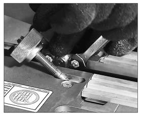
1. Using a 7 mm open end wrench, first remove emitter retention nut on spring tensioner side of machine. A Belleville washer resides between retention nut and emitter. Use care to avoid dropping nut or Belleville washer into machine. If parts are dropped into machine, see "CLEANING OF MACHINE" below, for removal of fixed platen, to allow access to machine internals.
