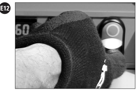
When machine cools to "splice start" temperature and light illuminates, immediately press green start button to initiate splice heating cycle. Closely attend machine during splice cycle.
