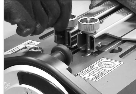
Install and tighten belt clamp bars, ensuring belt drive bars are fully seated in templates.
