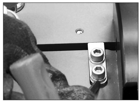
Move platen stop plate to contact fixed platen face. Repeat for platen stop plate on opposite end of platens – move to contact blade holder.
