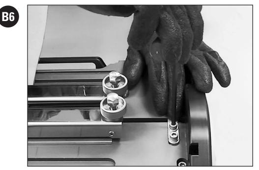
Tighten two socket head cap screws using 5 mm hex driver. Repeat for platen stop plate on opposite end of platens.
