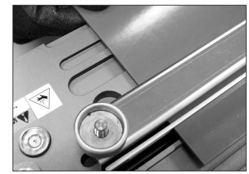
Ensure belt is positioned "square" to machine by either engagement of positive drive feature, or by using a square or alignment marks. **Note!** Belt should be centered in machine for splicing.
