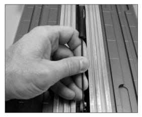
**11.** Remove guard. Using 2 mm ball driver, verify 2 mm clearance between emitter and thermocouple. This is the factory setting and should not change unless thermocouple is contacted during emitter replacement. Carefully adjust thermocouple only if necessary. Lightly press against thermocouple to adjust position. Thermocouple height is not adjusted.
