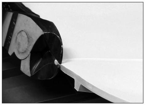
Trim splice weld bead from belt edges using Flexco Unibar cutter. **Note!** Spliced belt widths may vary. If necessary, cut taper lead on any edge, removing any "steps" from belt edges.
