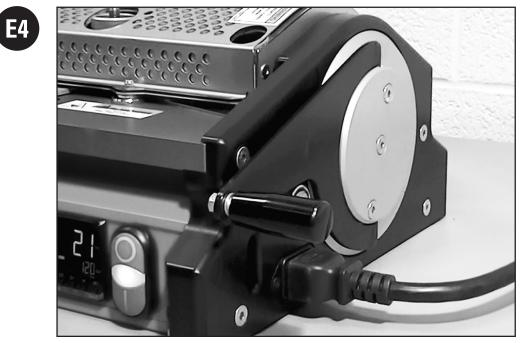
Open platens and raise emitter into heating position using actuator lever.
