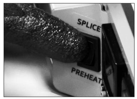
During this cooling period, set heating mode rocker switch to SPLICE position.
