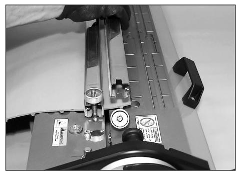
Loosely clamp remaining belt clamp bar. DO NOT TIGHTEN CLAMP BAR. This clamp bar is installed to provide protection from cutter blade. It is important that belt relief is allowed on loosely clamped side of cutting blade during cutting process.
