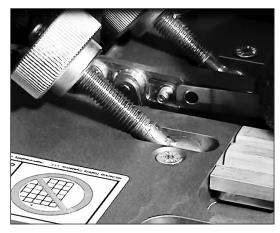
**2.** Once emitter retention nut and Belleville washer are removed, manually compress emitter spring tensioner and disengage emitter from emitter block retention stud.
