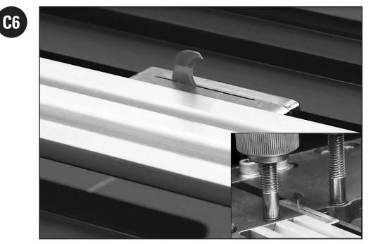
Drive cutter blade to machine side opposite controls. **Caution!** Use cut resistant gloves during cutting operation. Ensure blade is parked at full travel position of cutter, between clamp studs.
