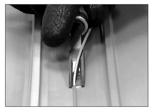
Remove underside weld bead with skiving tool.
