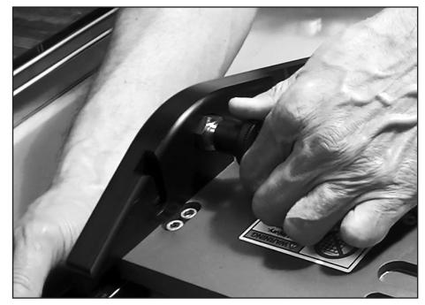
Lock in place with locking pin.
