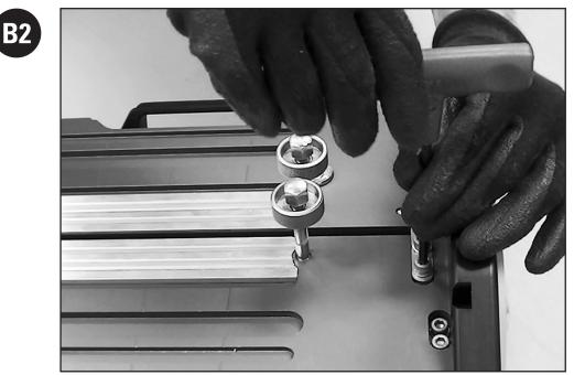
On platen stop plate, loosen two socket head cap screws using a 5 mm hex driver. Repeat for platen stop plate on opposite end of platens.
