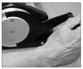
6. Rotate actuator lever/cam disk to close platens.
