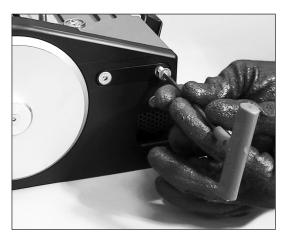
**1.** Loosen and remove four (4) platen locking screws.
