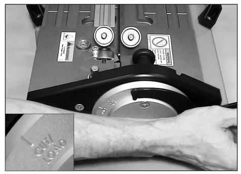
Rotate lever to cut/load position.
