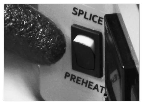
Place heating mode switch to PREHEAT position.
