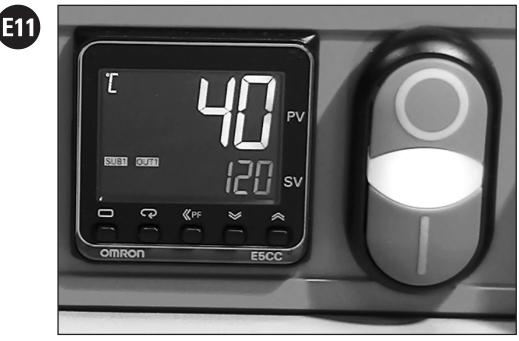
Factory preset "splice start" temperature is 40°C. A white light on start/stop switch will illuminate when control temperature is at or below setting.
