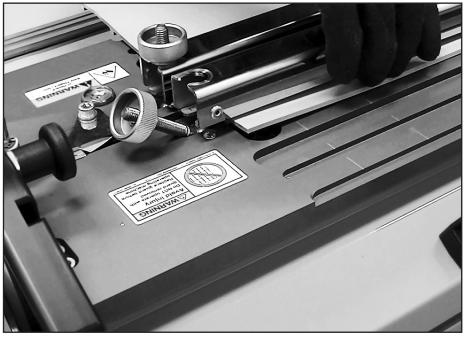
Relax clamp thumb nuts and remove clamp bars. Move prepared belt end clear of machine.
