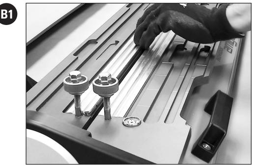
Ensure template and platen receiving slots are clean and debris free. Templates are directional and are keyed to fit in the proper direction. Insert outside edge first, push down on inside edge to secure in place.
