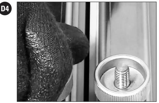
Clamp prepared belts in machine using clamp thumb nuts, ensuring uniform clamping pressure across belt width.
