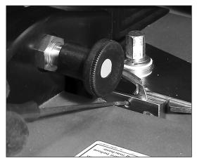
2. Using the 2 mm ball driver provided, loosen blade retention set screw 1 turn MAXIMUM. Caution! DO NOT loosen excessively. Set screw is very short and can become disengaged and lost.
