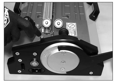
Engage cutter crank with cutter drive shaft.
