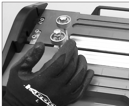
15. Move fixed platen lightly against blade holder.
