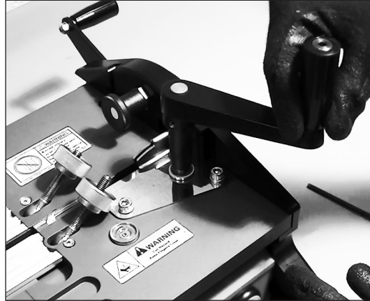
11. Crank blade holder just outside of stowed area.
