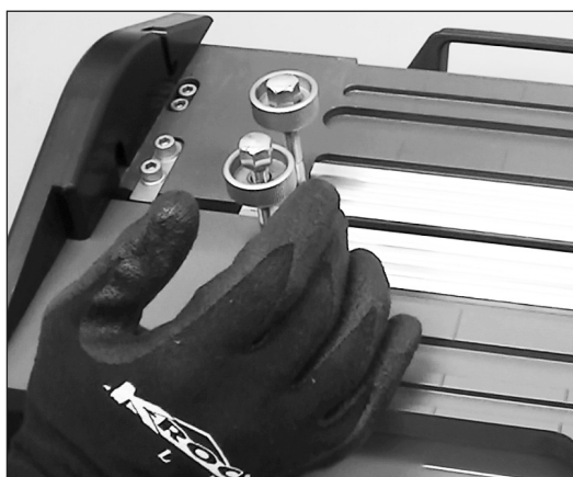
15. Move fixed platen lightly against blade holder.
