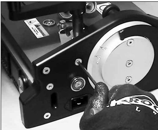
18. Loosen two (2) platen locking screws at control end.
