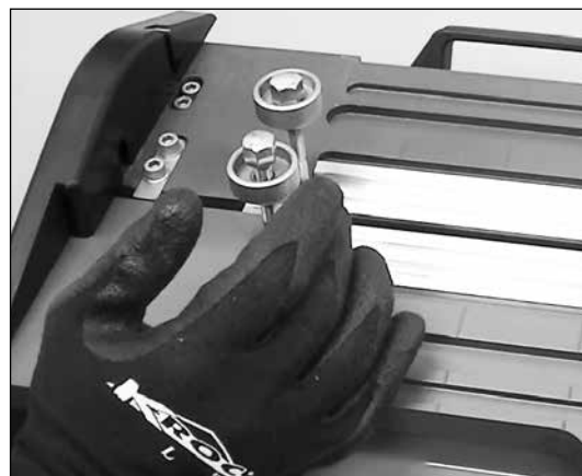
15. Move fixed platen lightly against blade holder.
