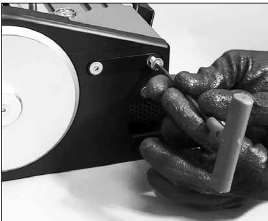
1. Loosen and remove four (4) platen locking screws.
