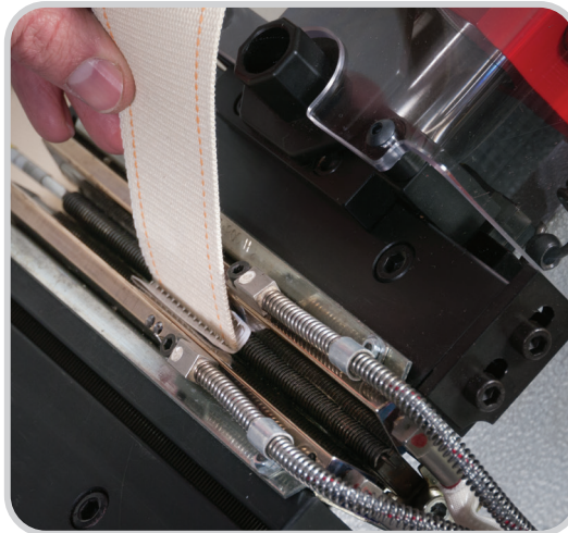
Built-in cooling station insures proper bonding of the patch material with the laundry tape
