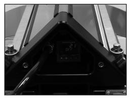
13. Place 0.5 mm silicone cloth (or silicone matrix pad) on top of prepared splice. Install Aero<sup>™</sup> Press upper beam, attaching it to lower beam using connecting bolts.
