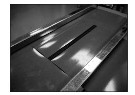
12. Place 3 mm silicone pad onto lower platen of Aero<sup>™</sup> press. Trim ASL ends to be flush with belt edges. Place prepared ASL splice, conveying side upwards, onto 3 mm silicone pad. Fix belt in this position using Aero Belt Clamps. Fill balance of press width with belting.
