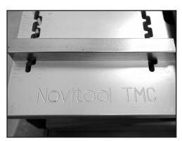
6. Using the Novitool Ply 130<sup>™</sup> to prepare the belt ends, set the belt guide to the appropriate position as indicated in the below chart.
