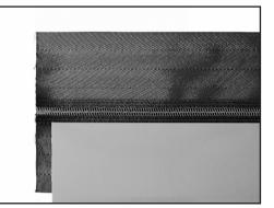
9. Insert the fabric side of the adhesive-primer coated ASL, between the separated fabric plies. ASL fabric overlap should be upwards, towards the conveying side. The ASL should extend somewhat past each side of the belt. Insertion should be to a depth where the belt ends extend to the ASL stitch line, furthest from the spiral loop.
