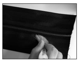
**4.** Using application brush, apply a thin coating of the prepared adhesive-primer to top and bottom ASL fabric. Apply adhesive primer up to stitch lines nearest spiral loop, keeping spiral loop area free from adhesive primer.
