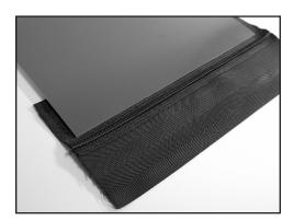
1. Cut belt ends square, yielding a belt length approximately 15 mm shorter than required finished length. Cut ASL to a length that is approximately 25 mm wider than belt width.
