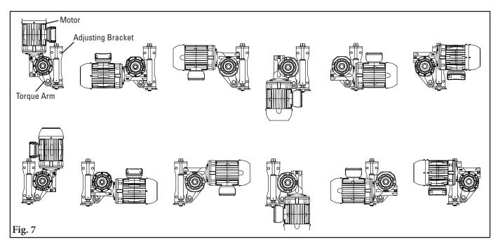
7. Determine desired motor mounting orientation. The motor can be mounted in any of the orientations shown below (Fig. 7).
