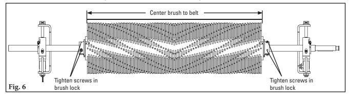
7. Set brush height. Turn adjustment nuts to raise brush until brush bristles just touch belt surface. The brush hub should now be 3-1/4" (83mm) below the bottom of the belt. Once bristles are touching belt, turn adjustment nut an additional 1-1/2 turns. The bristles should be compressed against the belt and brush hub should now be 3" (76mm) below the bottom of the belt (Fig. 7b). Place adjustment lock pins back into adjusting brackets.
