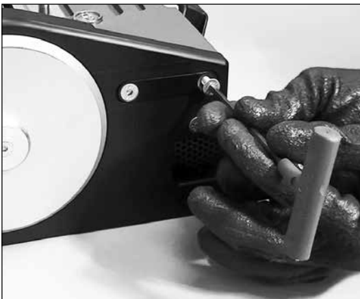
1. Loosen and remove four (4) platen locking screws.
