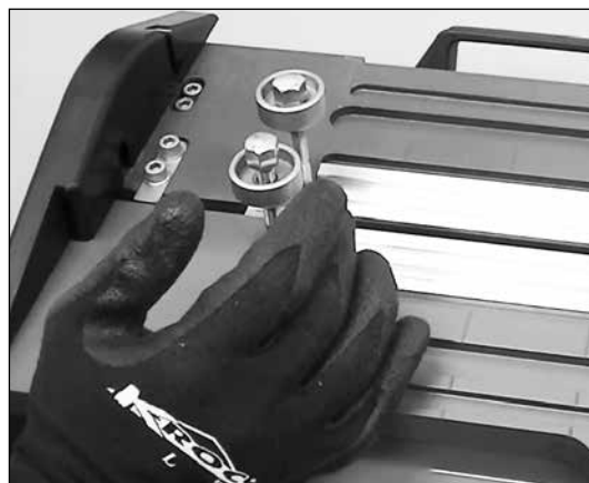
15. Move fixed platen lightly against blade holder.
