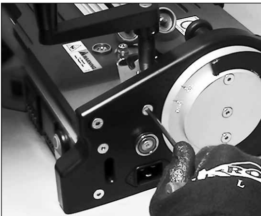
20. Fully tighten two (2) adjacent side platen locking screws.
