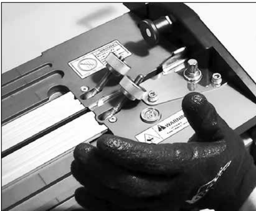
12. Move fixed platen lightly against blade holder.
