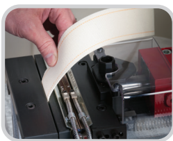
Built-in cooling station insures proper bonding of the patch material with the laundry tape
