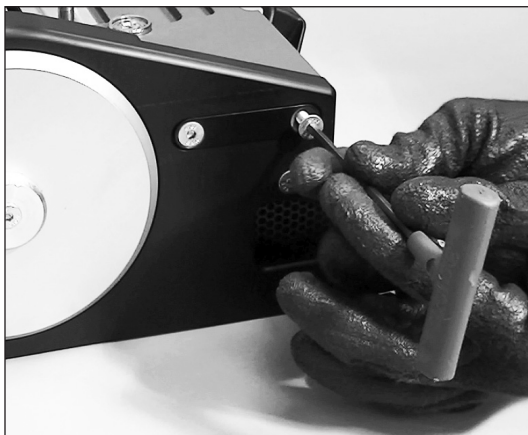
1. Loosen and remove four (4) platen locking screws.
