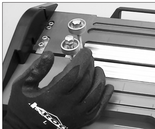
15. Move fixed platen lightly against blade holder.
