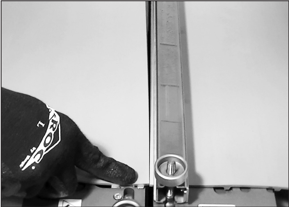
Load belt ends, aligning edges of prepared belt.
