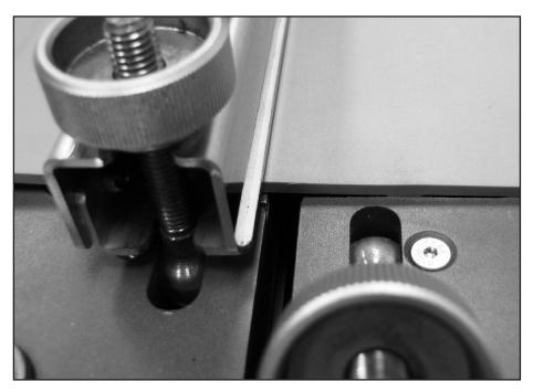
Clamp Bar orientation. "Balance" clamp load evenly when tightening clamp thumb nuts. This balanced load is particularly important when preparing tension-driven flat belt or belt possessing separated drive features. ALWAYS TEST FOR UNIFORM CLAMPING by pulling the belt. If belt slip is observed, readjust clamping thumb nuts to balance load. Clean friction tape surface as required assist in preventing slip.
