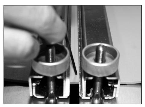
Using 2 mm ball driver provided, or an alternate "probe," determine by feel if prepared belt ends are uniformly aligned "vertically." No "step" should be felt when moving probe across cut length. If a step is recognized, attempt alignment of belt surfaces via tightening (or loosening) clamp thumb nuts.
