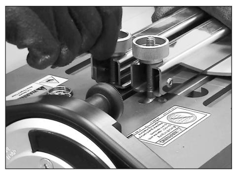
Install and tighten belt clamp bars, ensuring belt drive bars are fully seated in templates.
