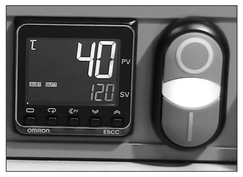
Factory preset "splice start" temperature is 40°C. A white light on start/stop switch will illuminate when control temperature is at or below setting.
