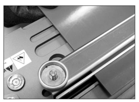
Ensure belt is positioned "square" to machine by either engagement of positive drive feature, or by using a square or alignment marks. **Note!** Belt should be centered in machine for splicing.
