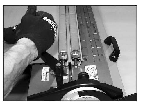
Using cutter crank, apply consistent cranking speed to draw cutting blade toward control end. **Important!** Do not stop cutting action, particularly when blade is entering or exiting belt. Failure to comply will result in an uneven cut.
