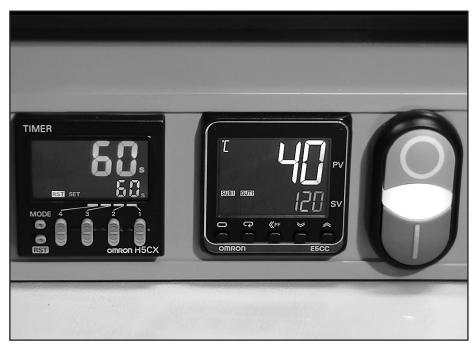
Allow machine to cool until white light illuminates (factory setting 40°C control temperature). **Warning!** Guard, clamp bars, and clamping thumb nuts are hot after splicing. It is important for safety and for splice integrity that the machine is allowed to cool after splice is made.
