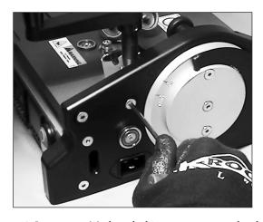
18. Loosen two (2) platen locking screws at control end.
