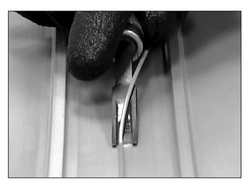
Remove underside weld bead with skiving tool.
