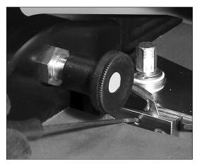
5. Ensure blade is properly seated in blade holder. Tighten blade retention set screw.
