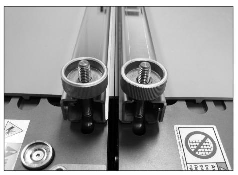
Position actuator lever to permit prepared belt ends to abut. There should be no more than approximately 0.1 mm (.004") gap along entire abutted faces. If gap is greater or uneven, it may be necessary to reprepare belt ends.
