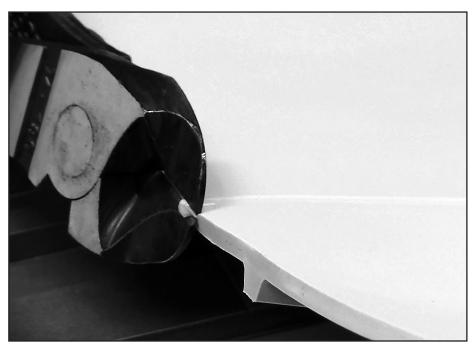
Trim splice weld bead from belt edges using Flexco Unibar cutter. **Note!** Spliced belt widths may vary. If necessary, cut taper lead on any edge, removing any "steps" from belt edges.
