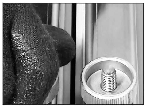
Clamp prepared belts in machine using clamp thumb nuts, ensuring uniform clamping pressure across belt width.
