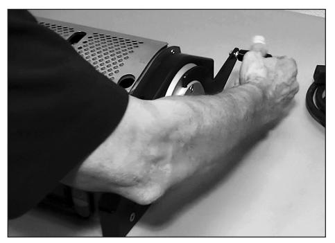
Rotate actuating lever to its operating position.
