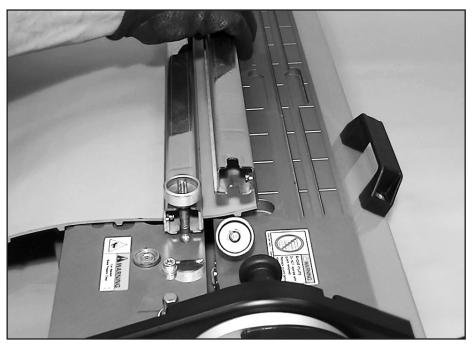
Loosely clamp remaining belt clamp bar. DO NOT TIGHTEN CLAMP BAR. This clamp bar is installed to provide protection from cutter blade. It is important that belt relief is allowed on loosely clamped side of cutting blade during cutting process.
