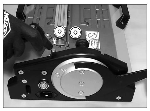
Engage cutter crank with cutter drive shaft.
