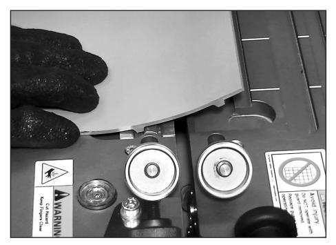
Engage belt with template. Position to cut out a problem belt area, or to simply prepare belt end with a precise cut for splicing. Belt must fully cover gap between platens. **Note!** Only belt ends prepared with the integrated cutter are sufficiently accurate to accommodate splicing.
