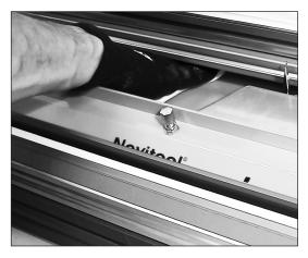
7. Raise emitter to access beneath sliding platen for cleaning opposite side. Lower emitter after cleaning.
