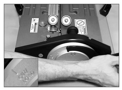
Rotate lever to cut/load position.
