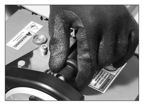
With both prepared belt ends clamped in machine, pull out and rotate locking pin to release it from locked position. **Note!** The pin is positioned as to not restrict actuator lever movement during splicing.
