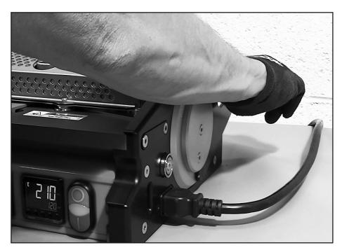
An audible signal tone marks the conclusion of the splice heating cycle. Immediately (within 1 second) at tone, rotate actuator lever to splice position and hold for approximately 5 seconds. Do not force actuator lever against internal stop.
