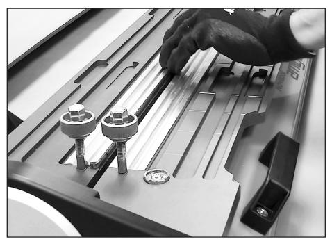
Ensure template and platen receiving slots are clean and debris free. Templates are directional and are keyed to fit in the proper direction. Insert outside edge first, push down on inside edge to secure in place.
