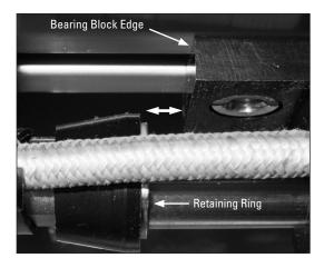
1. End-of-Emitter-Life retaining ring aligned with bearing block edge, when emitter is cold. Inspect emitter life indication in a "cold", power-off state. Image shown indicates significant emitter life remains. Emitter is at the end of its useful life when the "arrow" dimension is zero. Emitter must be replaced when the Retaining Ring is even with the Bearing Block Edge shown—in a cold, power-off state.
