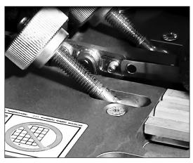
**2.** Once emitter retention nut and Belleville washer are removed, manually compress emitter spring tensioner and disengage emitter from emitter block retention stud.
