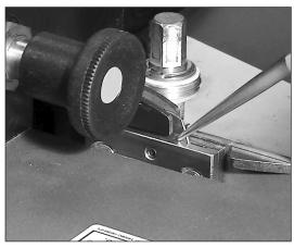
3. Using pliers, remove blade from blade holder.
