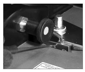
2. Using the 2 mm ball driver provided, loosen blade retention set screw 1 turn MAXIMUM. Caution! DO NOT loosen excessively. Set screw is very short and can become disengaged and lost.
