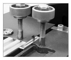
**14.** Crank blade holder fully to opposite side of machine.
