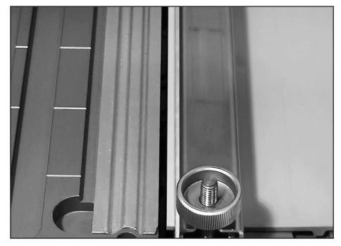
Ensure appropriate matched set of templates are installed in machine.
