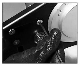
**13.** Lightly tighten two (2) adjacent side platen locking screws.
