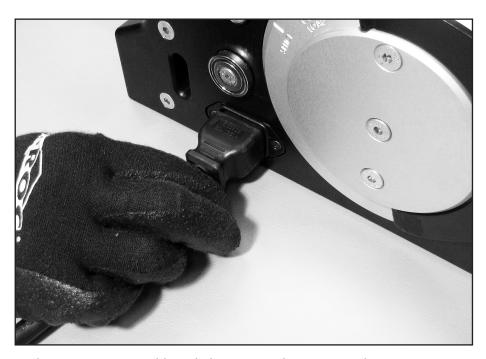
Select proper power cable and plug into machine power inlet.
