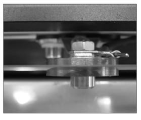
**9.** Ensure emitter is positioned on (or over) emitter support roller. **Note!** Emitter may possess a slight "bow" thus preventing initial contact with support roller. This will relax after several conditioning heat cycles. Ensure emitter is not in contact with thermocouple.
