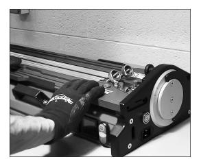
10. Lock actuating disc in cut/load position.
