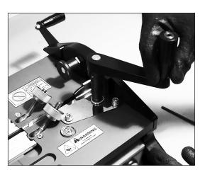
11. Crank blade holder just outside of stowed area.
