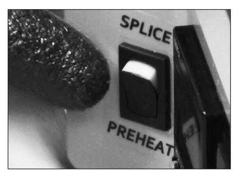
Place heating mode switch to PREHEAT position.
