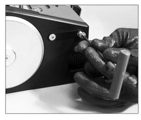
**1.** Loosen and remove four (4) platen locking screws.
