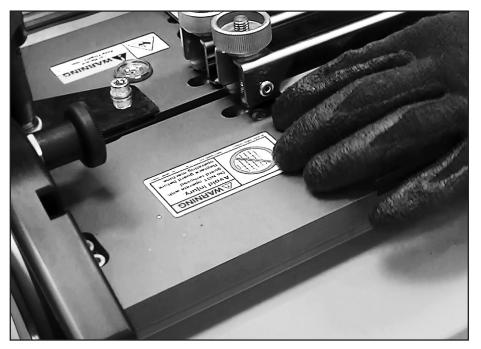
Support belt to prevent belt from "peeling away" during cutting. Failure to comply will result in an uneven cut where blade exits from belt. TIGHTLY CLAMPED side of belt is now prepared for splicing.
