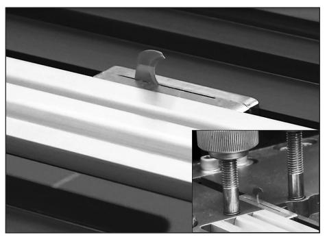
Drive cutter blade to machine side opposite controls. **Caution!** Use cut resistant gloves during cutting operation. Ensure blade is parked at full travel position of cutter, between clamp studs.
