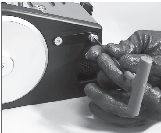
1. Loosen and remove four (4) platen locking screws.
