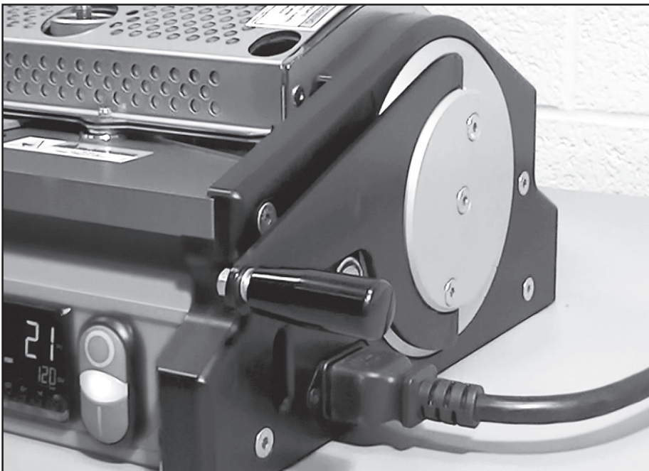
Open platens and raise emitter into heating position using actuator lever.
