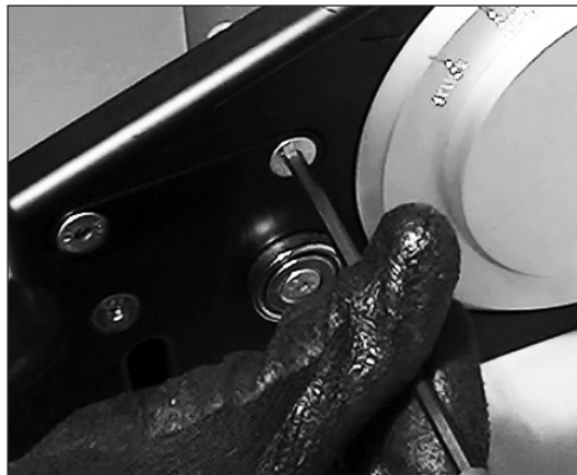
13. Lightly tighten two (2) adjacent side platen locking screws.
