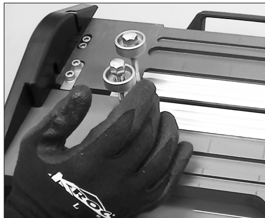
15. Move fixed platen lightly against blade holder.
