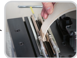
Heated jaws activate the glue during the quick installation process
