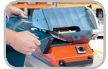
Separate up to 5" (130 mm) in a single pass
