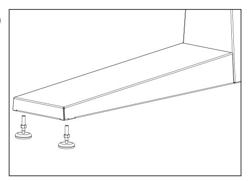
Ensure jam nuts are positioned onto the threaded shafts of the leveling feet (as shown) before installation. Install two leveling feet (item # 7.1) into Aero Stand base (item # 3). Ensure leveling feet are fully engaged through mounts.
