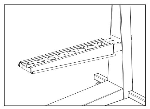
Using six M8  $\times$  20 mm screws (item # 7.3) assemble cradle (item # 4) to column assembly (item # 1) **Note:** Install all screws intially loose, tightening after all are installed.
