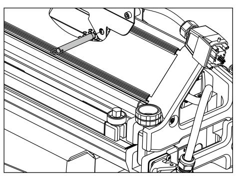
Load the upper beam of the Aero Press onto the lower beam. Use the detent pins (item #7.2) to connect the lifting interface to the top of the Aero Press upper beam. Ensure the press is centered under the lifting cables.
