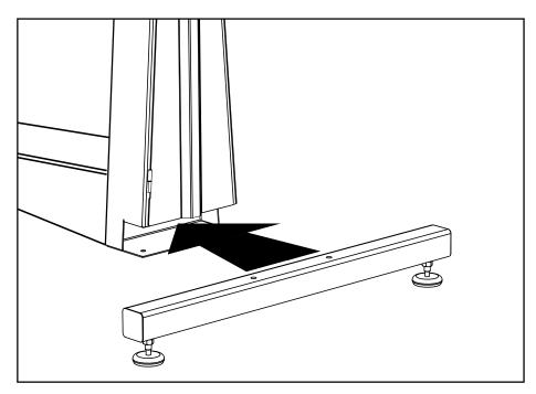
Using two M12  $\times$  100 mm bolts (item # 7.6) and two M12 nuts (item # 7.5) assemble cross support assembly (item # 6) into column assembly (item # 1).
