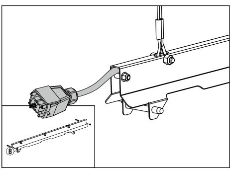
With Aero Stand 08114, use two M6  $\times$  30 mm screws (item # 7.7), two M6 nuts (item # 7.9), and two 6 mm spacers (item # 7.10) to secure the umbilical cable extension (item # 08319) into the lifting interface, with non-latch connector extending from end B.
