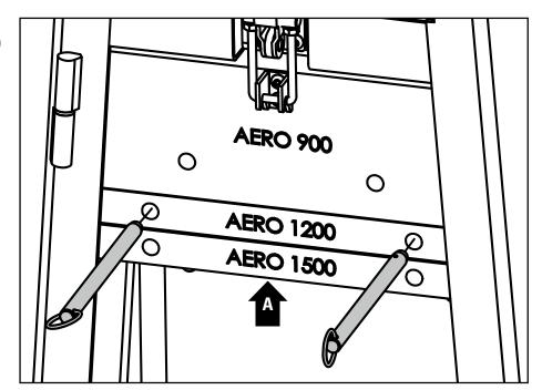
With an Aero 900 or 1200 loaded into the stand, ensure weight latch is engaged and support counterweights (position A) labeled AERO 1500 and 1200. Remove the pins from the Aero 1500 counterweight and install them into the counterweight corresponding with the Aero Press in the stand. Ensure both weight pins are completely engaged. Avoid pinch points within the weight path!
