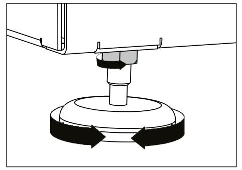
With the Aero Stand located for operation, rotate the leveling feet as necessary to be sure that the stand is level. Assure that the leveling feet shafts remains fully engaged through the frame. Tighten all leveling feet jam nuts to the frame.
