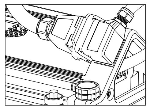
If using umbilical cable extension, secure the upper beam connectors to the top of the Aero Press with Velcro fastening strip.
