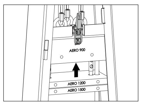
Raise the Aero 900 weight and engage the weight latch. Raise the Aero 1200 and 1500 weights and secure them in the uppermost position with the pins. Avoid pinch points within the weight path!
