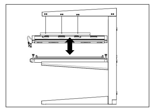
With the Aero Press upper and lower beams disconnected from each other, manually raise and lower the upper beam as needed for your splicing process.
