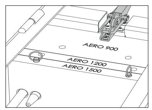
With column assembly laying on the floor, open door and remove packing material. Install pins in weight mechanism to Aero 1500 location. Slide all three weights to the top and fasten into place with the toggle clamp. Ensure that latch is secured to the weights.
