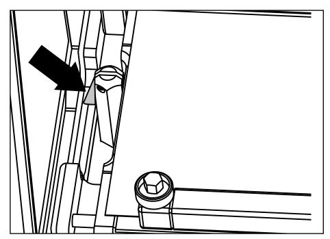
• Push down on the locating post latch, simultaneously lifting the lower beam of the Aero Press from the Aero Stand cradle. Avoid pinch points!
