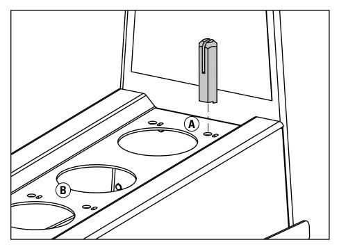
Install locating post (item # 7.13) into cradle (item # 4) using one M10  $\times$  20 mm screw (item # 7.12), inserted from below. Position A for Aero 1200 and 1500. Position B for the Aero 900. Post is keyed for proper orientation.
