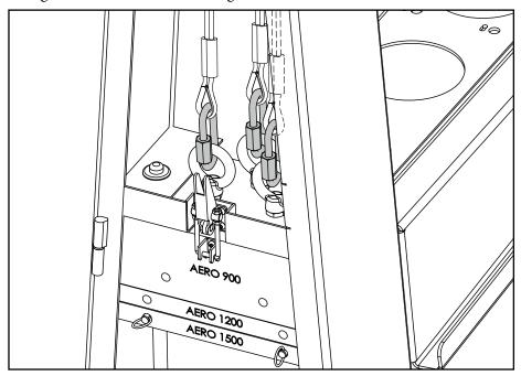
Follow the cables from the pulley located in the top beam from the back side of the Aero Stand assembly for proper positioning. Fix the cables to the weight system using the provided quick link clevises.
