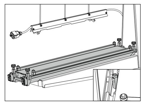
Place the lower beam of the Aero Press in the support cradle, with the locating post extending up through press handle opposite the control end. Avoid pinch point where locating post interfaces with the press.
