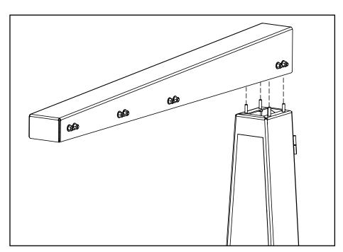
Using four M8  $\times$  30 mm screw (item # 7.4), install top beam assembly (item # 2) to column assembly (item # 1). **Note:** Install all screws initially loose, tightening after all are installed.
