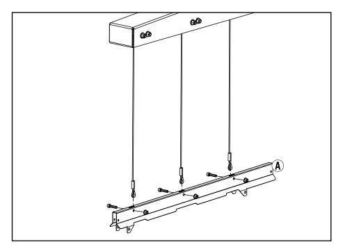
With longer extension (A) towards the column assembly, install lifting interface (item #5) to the three cables hanging from the top beam assembly using three M8  $\times$  35 mm screws (item # 7.8) and three M8 nuts (item # 7.11).
