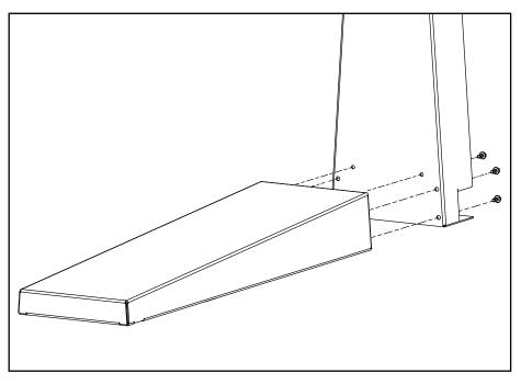
Using six M8  $\times$  20 mm screws (item # 7.3) assemble base (item # 3) to column assembly (item # 1). Note: Install all screws intially loose, tightening after all are installed.
