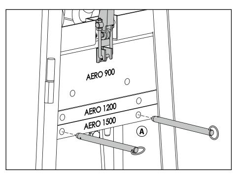
With the weight latch engaged, manually support the weights (position A), remove the pins and lower the weights, taking care to avoid pinch points. Support the remaining (Aero 900) weight (Position A), disengage the weight latch and lower the Aero 900 weight. Avoid pinch points within the weight path!
