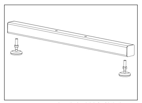
Ensure jam nuts are positioned onto the threaded shafts of the leveling feet (as shown) before installation. Install two leveling feet (item # 7.1) into cross support assembly (item # 6). Ensure leveling feet are fully engaged through the mounts.
