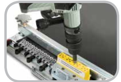
Electric Powered Rivet Driver Installation
