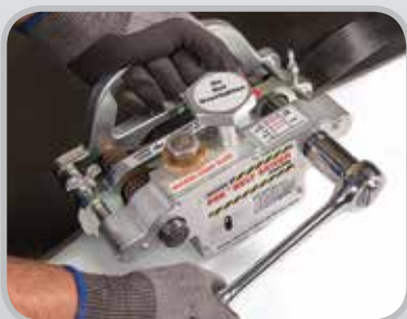
FSK™ Belt Skiver with metal fence
