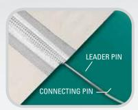
Connecting pin installation can be difficult, given both the small diameter of the pin and the flexibility of the material. To ease and speed this process we offer Leader Pins, which attach a smaller diameter, rigid lead pin to the larger diameter, flexible connecting pin. The lead pin is easily fed through the splice, allowing the actual connecting pin to be pulled through. The use of Leader Pins often reduces pin insertion time by more than 75%.
