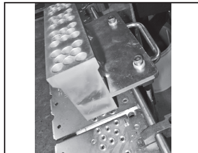
6. Check to make sure holes line up between guideblock and MSRT.
