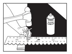
**NOTE:** The preferred method is to bore bolt holes using a power punch. A hammer and punch can also be used.
