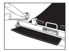
1. Square belt ends using centerline method. Cut belt ends using Flexco 840 Series Belt Cutter.
