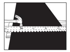
**2.** Support belt ends with a wood board. Align VP templet with belt end and align holes approximately 25mm (1") and equal distance from belt edges. Nail templet in position.
