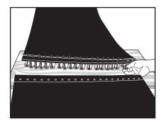
5. Insert bolts into holes in one belt end.
