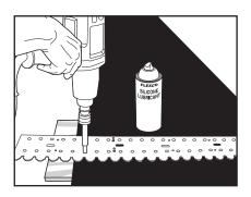
**3.** Spray templet holes with Flexco Silicone Lubricant. Bore bolt holes using an impact tool, quick change chuck, and power punch. Remove templet.
