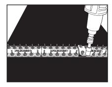
**10.** Tighten all nuts from edges to center. Tighten uniformly. Trim excess Flexco-Lok Tape.
