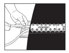
8. Cut Flexco-Lok<sup>\*</sup> Tape 3-½ times the belt width. Feed tape under top plates, under bottom plates, then back under top plates.
