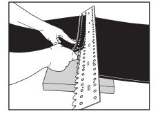
**6.** Align other bolts with templet teeth, then insert these bolts through holes in second belt end. Remove templet.
