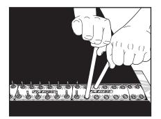
**11.** Break off excess bolt ends using Flexco Bolt Breaker.
