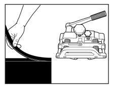
**4.** For belts with a top cover of 4.8 mm (3/16") or greater, skiving is highly recommended. Refer to the FSK<sup>™</sup> Belt Skiver instructions.
