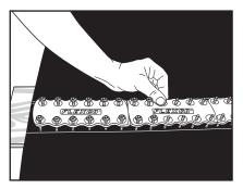
**7.** Place top plate strips over bolts using bolt horn. If shorter strips are needed, cut between plates with a utility knife. Start nuts on bolts.
