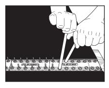
**11.** Break off excess bolt ends using Flexco Bolt Breaker.
