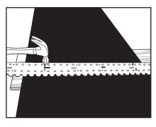
2. Support belt ends with a wood board. Align VP templet with belt end and align holes approximately 25mm (1") and equal distance from belt edges. Nail templet in position.
