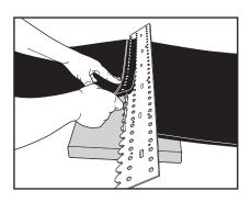
**6.** Align other bolts with templet teeth, then insert these bolts through holes in second belt end. Remove templet.
