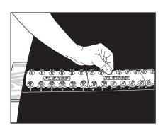
7. Place top plate strips over bolts using bolt horn. If shorter strips are needed, cut between plates with a utility knife. Start nuts on bolts.
