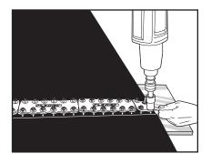
**9.** Pull tape tight and tighten nuts using Flexco wrench. **NOTE:** A Flexco Power Wrench and impact tool will speed this step. Max torque: 250 Lb-Ft (340 N-m).
