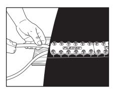
**8.** Cut Flexco-Lok® Tape 3-½ times the belt width. Feed tape under top plates, under bottom plates, then back under top plates.
