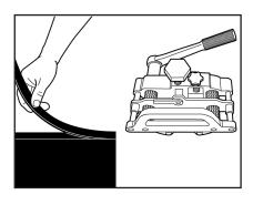
**4.** For belts with a top cover of 4.8 mm (3/16") or greater, skiving is highly recommended. Refer to the FSK $^{\sim}$  Belt Skiver instructions.
