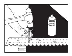
**NOTE:** The preferred method is to bore bolt holes using a power punch. A hammer and punch can also be used.
