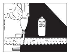
**3.** Spray templet holes with Flexco Silicone Lubricant. Bore bolt holes using an impact tool, quick change chuck, and power punch. Remove templet.
