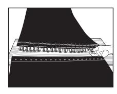
5. Insert bolts into holes in one belt end.
