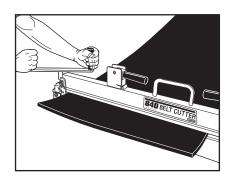
1. Square belt ends using centerline method. Cut belt ends using Flexco 840 Series Belt Cutter.
