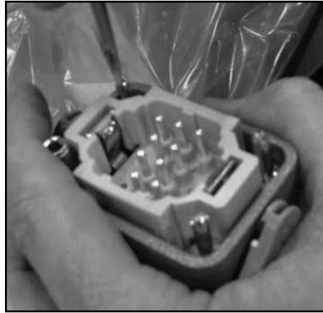
11. Line up the pins and bushings with the threaded holes in the housing. Tighten with a screwdriver. BE CAREFUL NOT TO OVERTIGHTEN.
