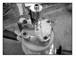
2. Using the 8 mm Allen wrench, loosen and remove the four M10-40 mm screws and flat washers that attach the Nose Assembly to the tool housing.
