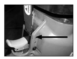
**10.** Reassemble the tool by repeating steps 1-8 in opposite order. \*\*Make sure to realign the safety mechanism while reattaching the Nose Assembly.\*\* Make sure to apply Loctite 242 or equivalent to the M10 screws and flat washers and torque to 50 ft/lbs.
