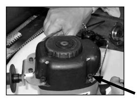
**6.** Remove Rear Housing: using the 6 mm wrench, remove the four screws from the housing. Set aside the handle and brackets before proceeding.
