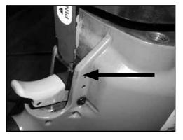
2. Reassemble the NEW Safety Trigger Spring (P3995) and Safety Trigger Assembly to the tool by reversing step 1 using Loctite 242 or equivalent and torque to 10-15 ft/lbs. \*\*Make sure to realign the safety mechanism while reattaching the Nose Assembly.\*\*
