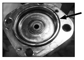
3. Remove the Nose Assembly from the tool. \*\*MAKE SURE O-RING IS ATTACHED TO THE BOTTOM OF THE NOSE ASSEMBLY\*\*
