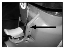
2. Reassemble the NEW Safety Trigger Assembly (N2292) with spring to the tool by reversing step 1 using Loctite 242 or equivalent and torque to 10-15 ft/lbs. \*\*Make sure to realign the safety mechanism while reattaching the Nose Assembly.\*\*
