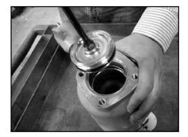
4. Remove Piston/Drive Rod Assembly from tool.
