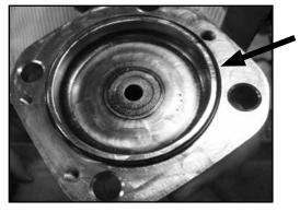
2. Remove the Nose Assembly from the tool. \*\*MAKE SURE O-RING IS ATTACHED TO THE BOTTOM OF THE NOSE ASSEMBLY\*\*
