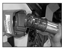
8. Grasp the rear portion of the cylinder and remove.
