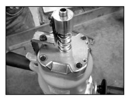
1. Using the 8 mm Allen wrench, loosen and remove the four M10-40 mm screws and flat washers that attach the Nose Assembly to the tool housing.
