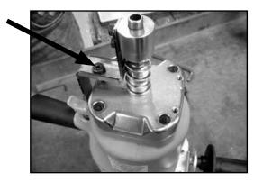
**1.** Using the 5 mm Allen wrench, loosen and remove the M6 Shoulder screw that attaches the Safety Trigger Assembly to the tool housing using hand pressure to hold the Safety Assembly down. Carefully remove Safety Assembly and spring to avoid any injury from the spring rebounding.
