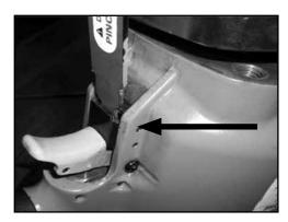
**5.** Reassemble the Safety Trigger Assembly to the tool by reversing step 1 using Loctite 242 or equivalent and torque to 10-15 ft/lbs. \*\*Make sure to realign the safety mechanism while reattaching the Nose Assembly.\*\*
