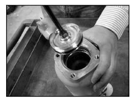
4. Remove Piston/Drive Rod Assembly from tool.
