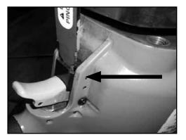
**5.** Reassemble the tool by repeating steps 1-3 in opposite order. \*\*Make sure to realign the safety mechanism while reattaching the Nose Assembly.\*\* Make sure to apply Loctite 242 or equivalent to the M10 screws and flat washers and torque to 50 ft/lbs.
