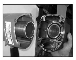
7. Carefully remove the Rear Housing and inspect for any debris.
