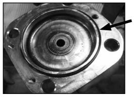
2. Remove the Nose Assembly from the tool. \*\*MAKE SURE O-RING IS ATTACHED TO THE BOTTOM OF THE NOSE ASSEMBLY\*\*
