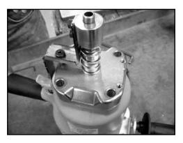
1. Using the 8 mm Allen wrench, loosen and remove the four M10-40 mm screws and flat washers that attach the Nose Assembly to the tool housing.
