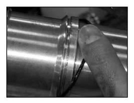
**9.** Replace with new cylinder P4149 along with the correct new "O" rings. If only replacing damaged "O" rings, then remove old "O" rings and replace with new ones from the "O" Ring Rebuild Kit (P4028). Reinstall the cylinder making sure to "seat" it at the nose of the tool.
