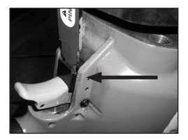
2. Reassemble the NEW Safety Trigger Spring (P3995) and Safety Trigger Assembly to the tool by reversing step 1 using Loctite 242 or equivalent and torque to 10-15 ft/lbs. \*\*Make sure to realign the safety mechanism while reattaching the Nose Assembly.\*\*
