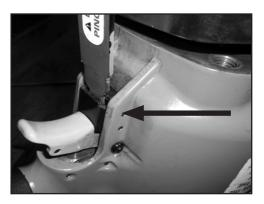
5. Reassemble the tool by repeating steps 1-3 in opposite order. \*\*Make sure to realign the safety mechanism while reattaching the Nose Assembly.\*\* Make sure to apply Loctite 242 or equivalent to the M10 screws and flat washers and torque to 50 ft/lbs.
