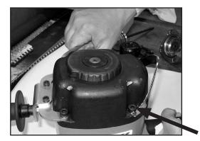
**6.** Remove Rear Housing: using the 6 mm wrench, remove the four screws from the housing. Set aside the handle and brackets before proceeding.
