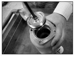
**4.** Remove Piston/Drive Rod Assembly from tool.
