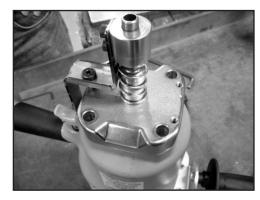
2. Using the 8 mm Allen wrench, loosen and remove the four M10-40 mm screws and flat washers that attach the Nose Assembly to the tool housing.
