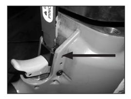
**5.** Reassemble the Safety Trigger Assembly to the tool by reversing step 1 using Loctite 242 or equivalent and torque to 10-15 ft/lbs. \*\*Make sure to realign the safety mechanism while reattaching the Nose Assembly.\*\*
