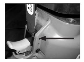
10. Reassemble the tool by repeating steps 1-8 in opposite order. \*\*Make sure to realign the safety mechanism while reattaching the Nose Assembly.\*\* Make sure to apply Loctite 242 or equivalent to the M10 screws and flat washers and torque to 50 ft/lbs.
