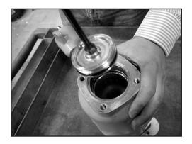
**4.** Remove Piston/Drive Rod Assembly from tool.
