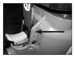
2. Reassemble the NEW Safety Trigger Assembly (N2292) with spring to the tool by reversing step 1 using Loctite 242 or equivalent and torque to 10-15 ft/lbs.
