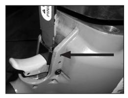
7. Reassemble the tool by repeating steps 1-4 in opposite order. \*\*Make sure to realign the safety mechanism while reattaching the Nose Assembly.\*\* Make sure to apply Loctite 242 or equivalent to the M10 screws and flat washers and torque to 50 ft/lbs.
