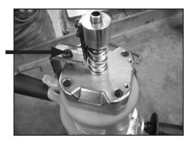
1. Using the 5 mm Allen wrench, loosen and remove the M6 Shoulder screw that attaches the Safety Trigger Assembly to the tool housing using hand pressure to hold the Safety Assembly down. Carefully remove Safety Assembly and spring to avoid any injury from the spring rebounding.
