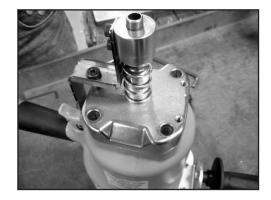
$\textbf{1.} \ Using the 8 \ mm \ Allen \ wrench, loosen \ and \ remove \ the four \ M10-40 \ mm \ screws \ and \ flat \ washers \ that \ attach \ the \ Nose \ Assembly \ to \ the tool \ housing.$
