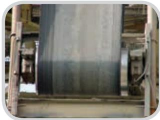
*Ensures center loading by installing before the tail pulley.*
