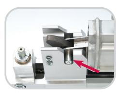
Allow the clamp beam to drop into position
