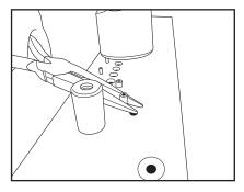
1. Insert 3/16" x 3/4" pin as shown. Hold pin with needle nose pliers. Gently tap pin in place until 1/4" remains above the tool surface.
