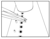
**2.** Insert 3/16" x 1/2" pin as shown. Hold pin with needle nose pliers. Gently hammer pin until .100" remains above the tool surface. Repeat for all pins this size.
