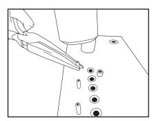
**3.** Insert 3/32" x 3/4" pins into the proper position as shown. Hold pin with needle nose pliers. Gently tap pin in place until .250" remains above the tool surface. Repeat for all pins this size.
